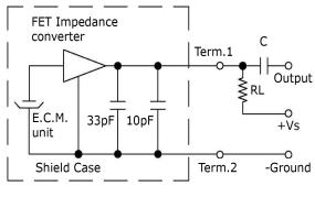
RL =  $2.2 \text{ k}\Omega$ C =  $1 \mu\text{F}$
