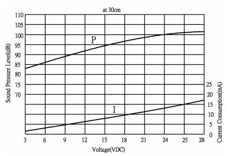
P: Voltage vs. Sound Pressure Level I: Voltage vs. Current Consumption
