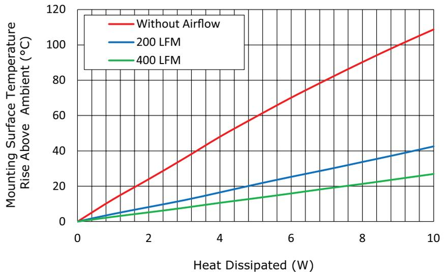
T<sub>hs</sub>: "hot spot" temperature measured on the heatsink
