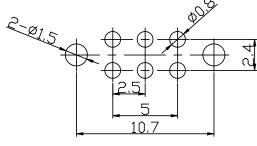
Recommended PCB Layout Top View
