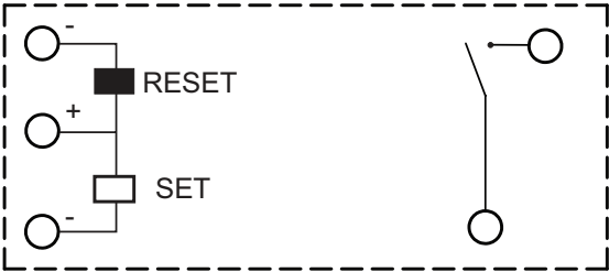
Wiring Diagram Bottom View
