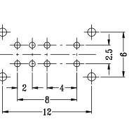
Recommended PCB Layout Top View
