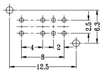
Recommended PCB Layout Top View
