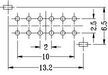
Recommended PCB Layout Top View
