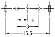
Recommended PCB Layout Top View
