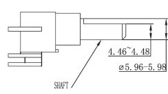
Compatible Shaft Size Withdrawal Force: 1.5~7.5 kg
