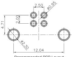
Recommended PCB Layout Top View
